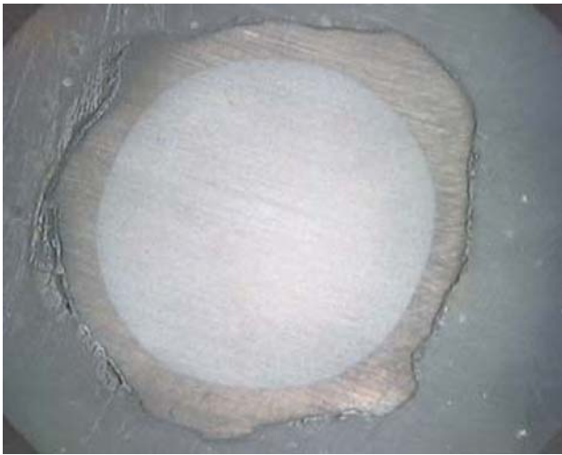
Fig. 1 Stereoscopic image of specimen cross section after Nital immersion
